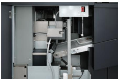
Uniquely designed delivery eliminates damage to the spine. Even 65 mm or 2.56" thick books or PUR bound books can be delivered without damage or marking.
