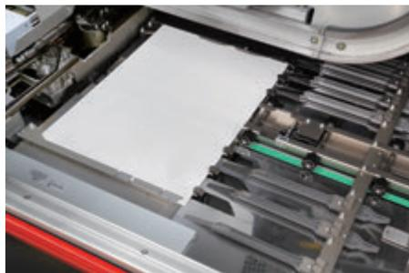
After transport to the nipping section, the cover is registered precisely with the fore-edge guide and tail-edge positioning guides.
