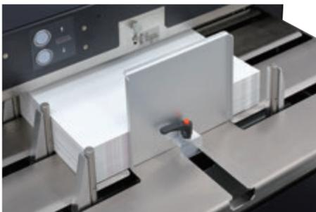
The high capacity cover feed station has a maximum pile height of 150 mm or 5.9" for continuous binding operation. The cover feeder can handle a wide range of covers: Bond Paper 81.4 to 302.4 gsm and Coated Paper 104.7 to 348.9 gsm.
