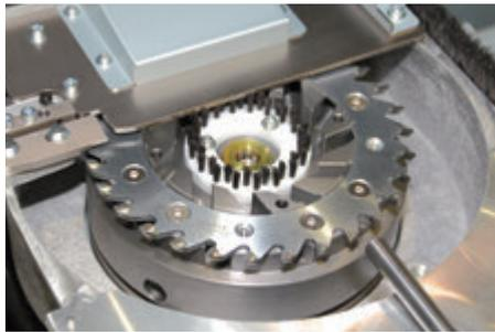
Powerful servo motor driven milling and notching mechanism mills the spine of the book block or signatures for optimum glue penetration and adhesion. Milling rotation speed can be adjusted automatically according to book thickness and custom templates. Milling depth can be adjusted from 0 to 4 mm or 0" to 0.157".
