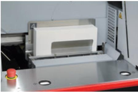
A rigid clamping system holds the book block firmly in position during the milling and nipping process to produce a quality finished book. The safety curtain ensures risk-free operation.
