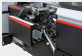
Install the special drain for glue run-off. The PUR tank and drums are tefflon coated so that the remaining glue can be easily peeled off after cooling.
