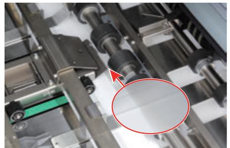
The scoring width and position are automatically set-up according to book block thickness and cover registration. Scoring is performed on thick covers for professional binding with sharp, square spines and hinge scores.
