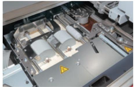
Dual application rollers and side gluing rollers ensure superior glue application to the spine and excellent adhesion of the cover for consistent quality binding. Glue roller height, wiper opening and cut-off timing, scraper roller height, and side glue roller width are automated.
